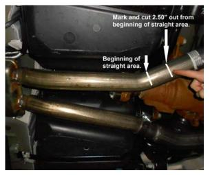
2) Begin by measuring back 2 <sup>1</sup>/<sub>2</sub>" from the beginning of the straight area shown in the photo at left and make a mark on both pipes. Support the exhaust system both in front and behind the area to be cut. Check that the marks are correct, then using a sawsall, cut both pipes at the marks. **Note: Due to the closeness of the pipes to the gas tank, use caution when cutting!** Carefully deburr the end of the muffler inlet pipes where cut with a file or die grinder.
