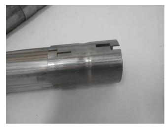
1) Slide the supplied **TB809S** adapter pipes onto the end of each outlet of the **86341S** X-pipe assembly. Place a supplied clamp onto the connections and tighten enough to hold.
