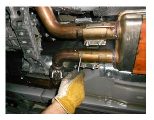
4) Loosen the four nuts at the two band clamp connections at the inlet of the center resonator. Using a screwdriver, pry up the clips on the clamp body to release the clip from the tab on the inlet pipes. Slide the clamp assemblies slightly back to clear the tabs. With the help of an assistant, carefully lower the stand and slide the assembly back to disengage from the inlet pipes.
