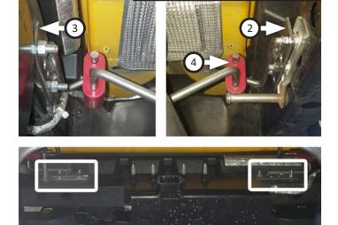
Connect muffler (1) to mid pipe, inserting wire hanger into rubber hanger. Adjust exhaust components for fit; maintaining 1/2" clearance and compensating for suspension, travel and vibration then tighten all clamps.
