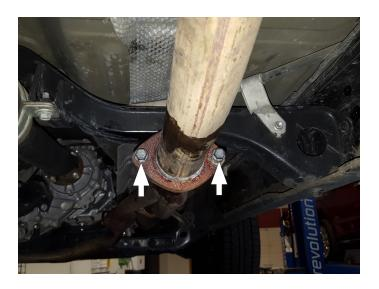
4. Disassemble factory exhaust wire hangers (x4) from isolators then remove system completely from vehicle.
