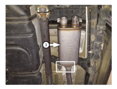
www.flowmastermufflers.com Technical Support (866) 464-6553 10. Route **right tailpipe (6)** and **left front tailpipe (4)** over axle and connect them to muffler outlets. Mount wire hangers into isolators then tighten clamps (x2) enough to allow for adjustment.
