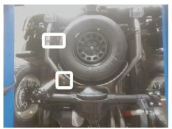
16. Adjust exhaust components for fit; maintaining ½" clearance and compensating for suspension, travel and vibration then tighten all clamps. Finally, fit (x5) hanger keepers (10) onto each sideways hanger.
