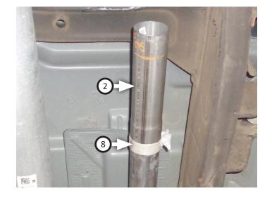
12. Place clamp (8) onto muffler (3) inlet. Place (x2) clamps (9) onto muffler outlets. Connect muffler to inlet or extension pipe then tighten front clamp just enough to allow for adjustment.
