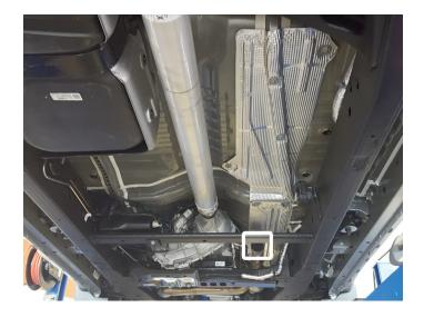
8. Release tab and remove factory clamp from pipe inlet. Retain factory clamp for later use.
