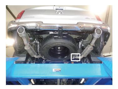
4. Remove factory tailpipe from vehicle by cutting it near muffler outlet and dismounting wire hangers from factory mounts.
