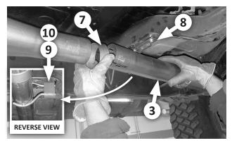
8. Install front hanger bracket (8) with 2 stock screws. Slip a 3" clamp (7) over extension pipe (3), slip the extension pipe over the headpipe, then install rubber hanger (9) on the bracket and pipe's hanger rods. Verify 3" of insertion, and snug the clamp slightly. Install the two 7/16" hanger keepers (10) on the hanger rods.
