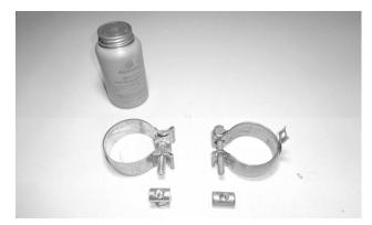
6. Before installing any clamps, remove their nuts, apply antiseize compound to the bolt threads, and re-install the nuts.
