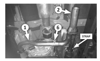
Slip a 2-1/2" clamp (6) over the head pipe assembly (2), slip the head pipe assembly over the left head pipe (1), then attach the pipes to the catalytic converter flanges using the stock gaskets and fasteners. (Reattach the bonding strap if applicable.) Verify 3" of insertion, and snug the clamp slightly (just enough to allow final adjustment later).
