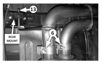
11. Slip two 2-1/2" clamps (6) over the muffler outlets. Insert both tailpipes in the muffler, and fasten the isolator mount to the frame using the stock screws. Verify 2" of insertion, and snug the clamps. Install the 1/2" hanger keeper (13) on the hanger rod.
