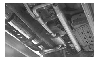
**13.** Adjust all components to give 1/2" to 3/4" clearance (about a finger's width) around them, and allowing for suspension travel and vibration. When you are satisfied with the system's clearance and fit, tighten all clamps.
