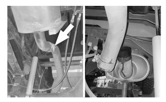
**2.** Loosen the clamp behind the muffler, and separate the tailpipe from the muffler.
