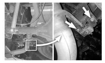
**3.** Remove the 2 screws from the tailpipe's isolator mount. Then remove the assembled tailpipe and mount from the vehicle.
