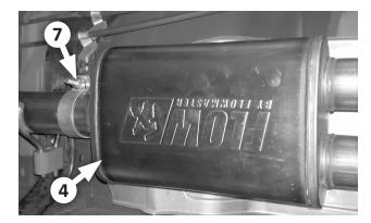
9. Slip the other 3" clamp (7) over the muffler's (4) inlet. Then install the muffler on the extension pipe and support it with a stand. Verify 2" of insertion, and snug the clamp.
