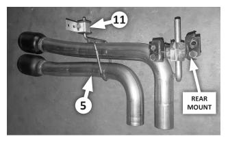
10. Install rear frame hanger (11) on the tailpipe assembly's
