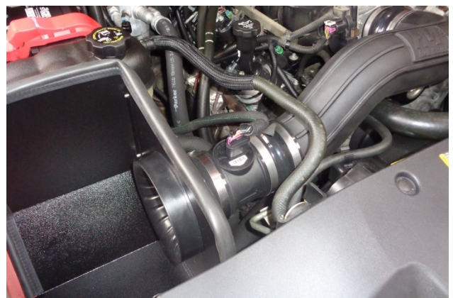
29. Plug the MAF sensor lead into the sensor until it clicks, then verify the connection is secure.
