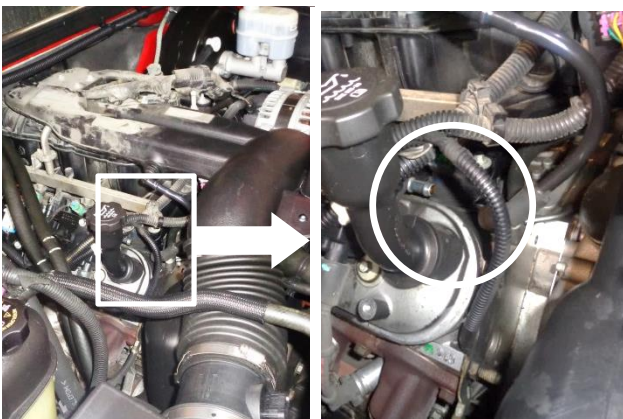
9. Carefully pull the breather hose off the breather line (just inboard of the oil filler neck – shown disconnected).
