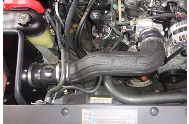
27. Adjust the intake tube as necessary to avoid contact with surrounding components (such as the radiator hoses). When the tube is aligned as desired, tighten the two tube clamps.
