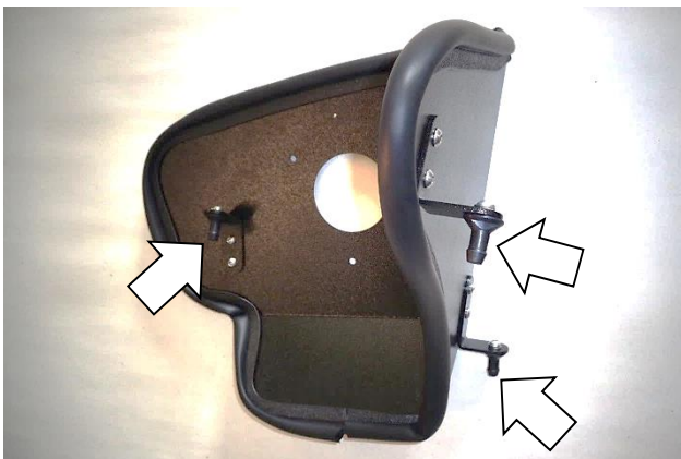
14. At each bracket, install barbed pin (6), using M6 screw (12), lock washer (10) and flat washer (8).
