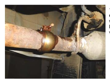
1) Locate the clamped connection just behind each of the factory exhaust tips, spray the clamp bolt with a penetrating lubricant and allow to soak. Loosen the bolts and remove the factory tips from the vehicle.
