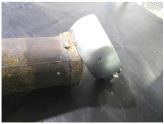
3) Place a factory clamp onto one of the new Flowmaster tips and put up into position behind the resonator on the right tailpipe. Tighten the clamp enough to hold the tip in place and adjust to the desired position. Tighten the clamp securely. Repeat this step on the left side of the vehicle.
