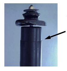
You must remove the rear shock, then, remove the upper mount to access the rear bump stop which is located underneath the OE dust boot
