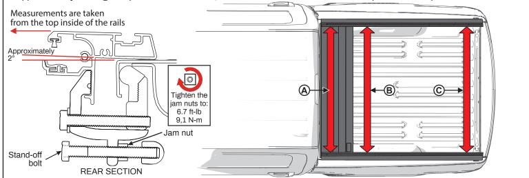
Remove the clamps (G) and turn the white adjustment screws with the 6mm Allen wrench (J) to move the rails. One complete turn = 1/16" (1.6 mm). Turn both screws. When properly adjusted, reposition and tighten the clamps as in steps 12-13, then proceed to step 16.
