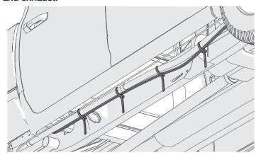
Insert a drain tube (D) into the cover **on both driver and passenger sides.** Rotate to the right; clockwise. The fitting will click twice when secure. Generally the drain tubes (D) will be routed out through a hole drilled in the factory bed plug, otherwise a suitable existing hole must be utilized. Alternately, a new hole can be drilled, but **take great caution to be aware of**
