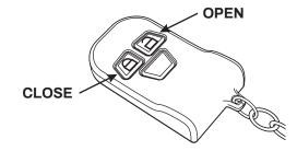
To enter "Cinch" mode to secure loose cargo in place against the tailgate, press the lock button three times. The cover will meet resistance and retract a couple inches. Press the lock button three times again and the cover will retract and cinch the object in place.
