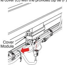
Go back underneath the vehicle where the main wiring harness (E) was zip-tied and pull out all the extra slack in the harness. Neatly organize and secure the extra slack, using another zip tie (F). **Keep the wires away from moving parts and exhaust.**
