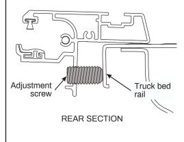
If the rails measure to be too close together, turn the screws counter clockwise.
