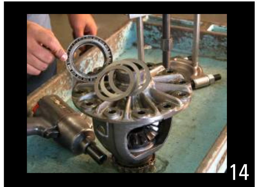
Make note of the shims by tagging them and keeping together for proper reinstallation. Bearings and shims from flange side shown.
