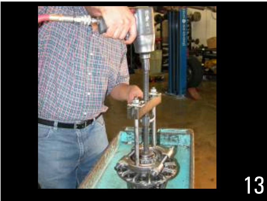
Remove bearings with bearing puller.
