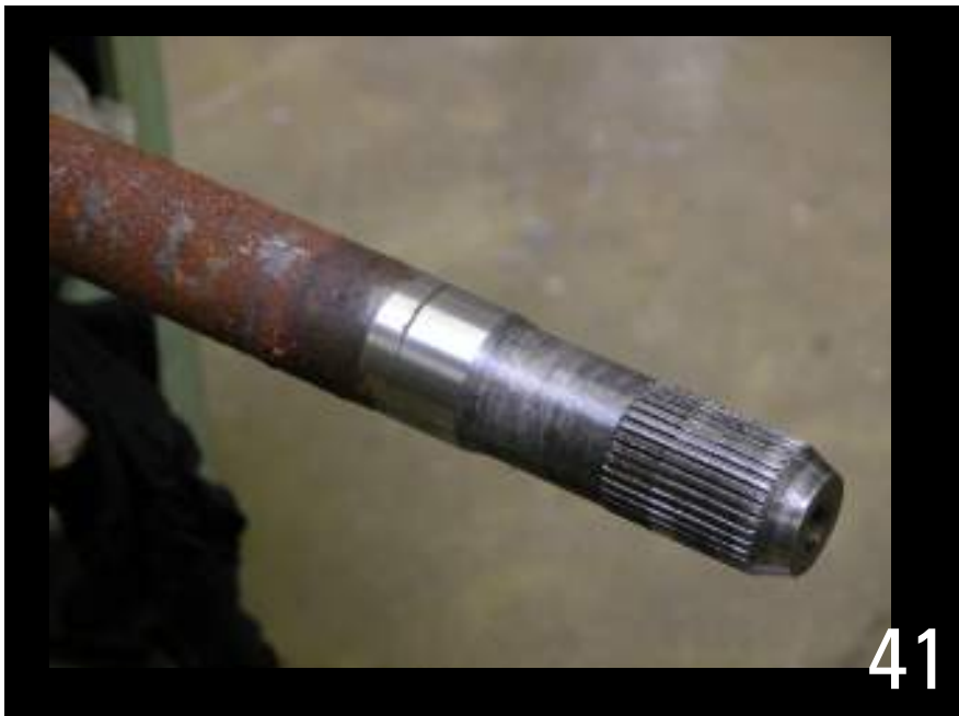
Clean axle shaft splines.
