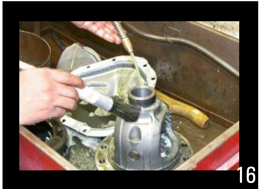
Wash the differential case, ring gear, ring gear bolts and other parts with nonflammable solvent.
