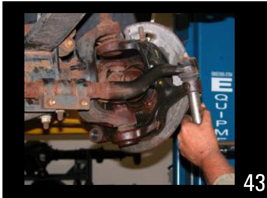
Reinstall tie rod end and torque to specifications.
