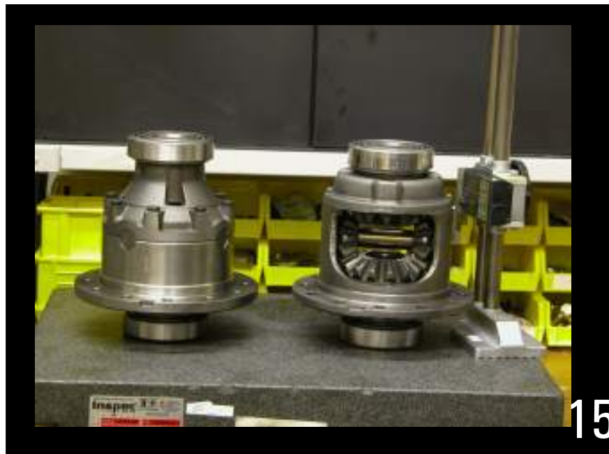
Measure the new Eaton differential case from precision (base) plate to the top of the bearing shoulder.
