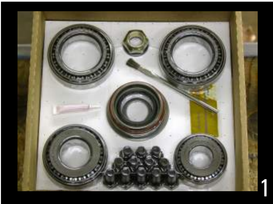
Prior to installation, be sure to have all of the proper installation components necessary for the job.
