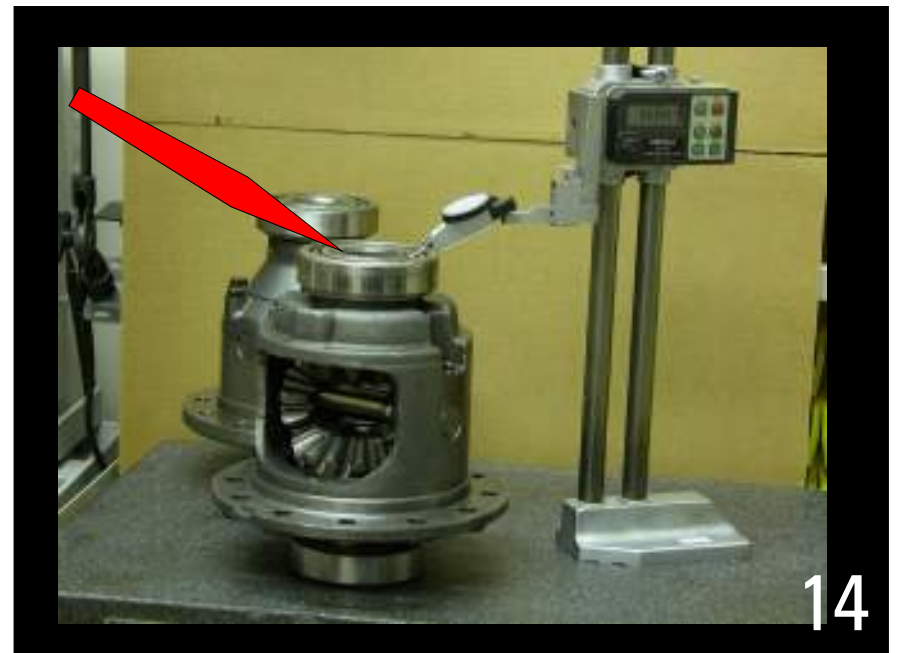
And from precision plate to top bearing shoulder.
