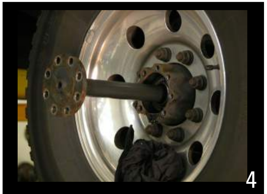
When removing axle shafts, do not allow the full weight of the axle to drag or rest on the axle seals. Inspect axle seals for wear.
