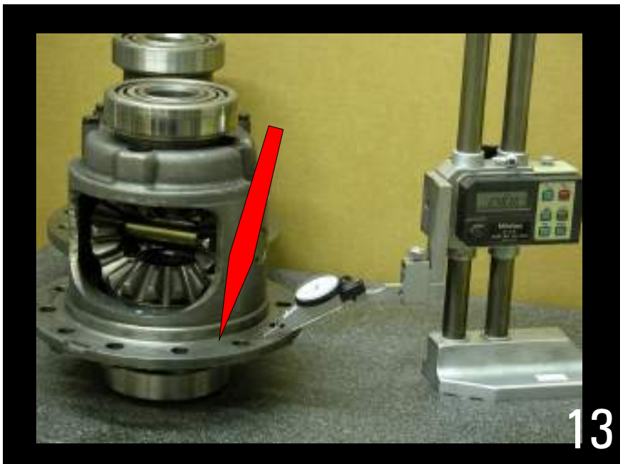
Measure the original differential case from precision (base) plate to ring gear flange. Please note that set up bearings (or equivalent) must be used to obtain an accurate measurement.
