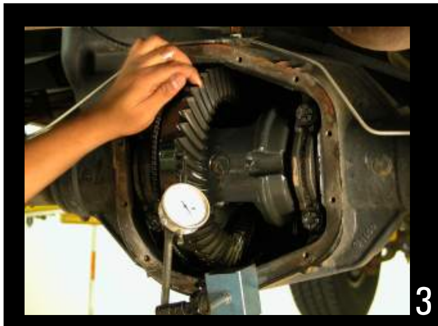
Measure the backlash from three equal places around the ring gear. Record measurements (if reusing ring and pinon set).
