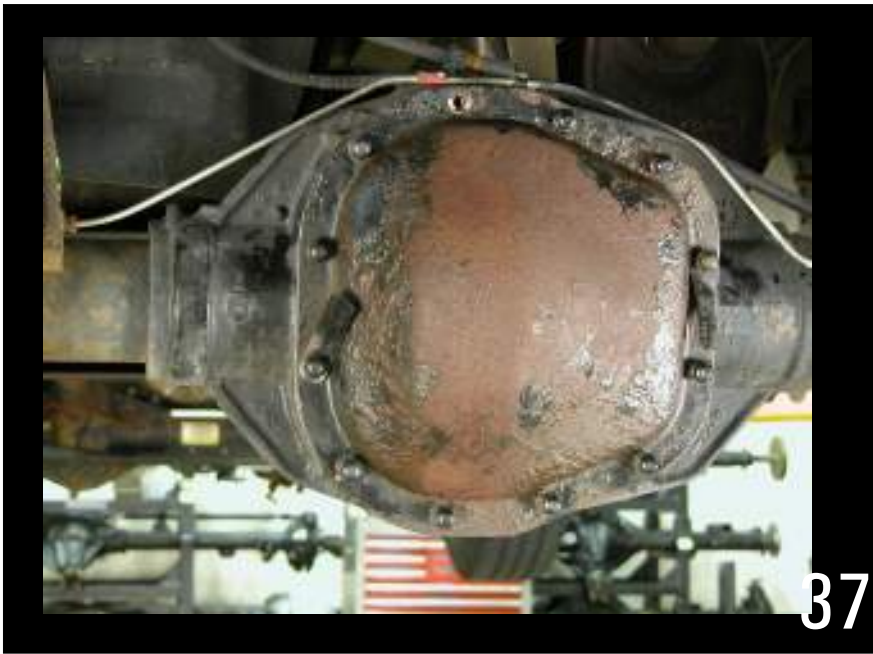
Install differential cover.
