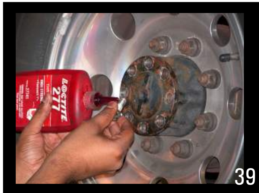
Use Loctite to hold hub bolts in place.
