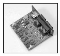
6) Install analog board. Analog board is supplied with two mounting legs. Install legs into main circuit board. Support analog board on ends near mounting legs, align legs with holes in board and pins to socket connector. Apply lite pressure to analog board until board is fully seated on legs and tangs are exposed.
