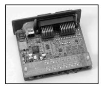
7) Apply a small amount of silicone sealant to case flange surface and slip board assembly back into case. Reinstall phillips head screws.
