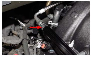
41. Install the provided fuel rail crossover to the 3/8" male fittings installed during step #40.
