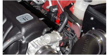
43. On 5.7L and 6.1L engines, reinstall the factory or factory replacement air intake system. **NOTE:** 6.4L engines require a factory or factory replacement 6.1L intake system.
