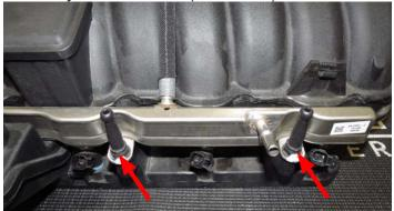
15. Firmly lift up on both sides of the factory fuel rail assembly to disengage fuel injectors from the intake manifold. In a gasoline safe container, empty the remaining fuel from the rails.
