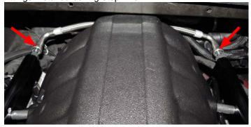
42. Lubricate the O-ring with silicone lube and install the provided -6 AN fuel rail plug into the front of the driver side fuel rail. Tighten until the hex makes contact with the rail.
