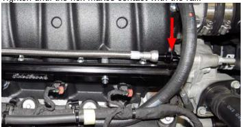
39. Connect the provided fuel input line from the factory fitting on the fire wall to the 180° fitting installed during step #38.
