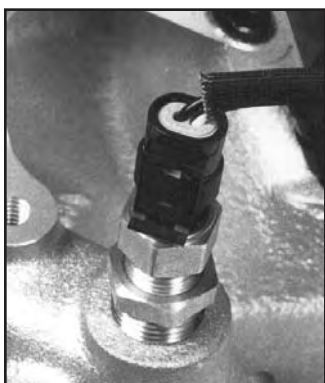
The Coolant Temperature sensor attaches to the harness with Connector J15.
