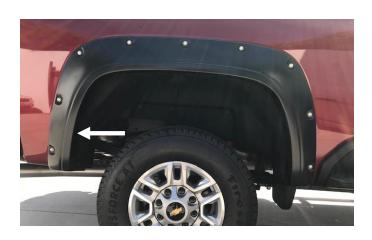
**STEP 12:** Place Fender Flare on the vehicle into the position of best fit. Note where the slot in Fender Flare aligns with the previously removed factory screws in the front and rear spats (steps 10 & 11). Using #15 Torx head screwdriver re-install the screws (H & I) from the rear factory spat through the slots in the Fender Flare.
