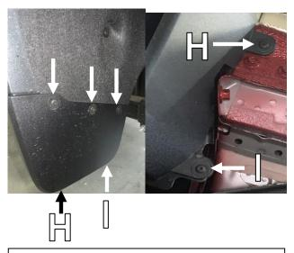
**STEP 11:** Using #15 Torx head screwdriver remove the two bottom screws (H & I), from the rear factory spat. Maintain screws for re-install.
