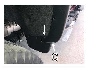
**STEP 14:** Using #15 Torx head screwdriver reinstall the previously removed factory mudguard screws at the upper and lower (G) screw locations through the slots in the front of the Fender Flare at the two noted locations.
