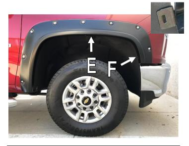
**STEP 6:** At the noted **E & F** positions, secure the Fender Flare to the wheel arch by ensuring the notch in clip locates securely into the slot in the Fender Flare.
