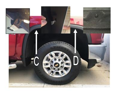
**STEP 5:** Using #15 Torx screwdriver remove factory screws at location **C** and **D**. Place Fender Flare on the vehicle into the position of best fit. Note where the slots in Fender Flare at positions **C**, **D**, and vehicle wheel arch are located. Install the large clips to the inner wheel arch by sliding clips into the Fender Flare slots, ensure notch in the clip locates securely into the Fender Flare slot. Re-install the factory screws through the hole in the clips to the wheel arch.
