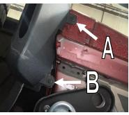
**STEP 4:** For models <u>with front</u> factory mud guards, remove factory Torx screw using #15 Torx head screwdriver at the upper and lower (**A** and **B**) screw locations (x 2). Maintain #15 Torx head screws for later reinstall. Remove the factory mud guard and discard, fender flares require the mud guards to be removed.
