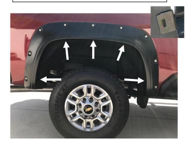
**STEP 13:** To secure the Fender Flare to the body, apply upward tension on Fender Flare to the vehicle fender when installing the black metal clips. Slide the clips over the Fender Flare and the inner wheel arch lip in the five locations shown. Position the clip so that the barb in the clip locates in the slot of the Fender Flare. Ensure all fixing points are tight and secure and that the rubber seal is flush neatly against the vehicle body. Repeat install steps for the opposite side.
