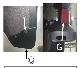
**STEP 10:** Using #15 Torx head screwdriver remove the upper and lower (**G**) screws from the front factory spat in the rear wheel arch. Maintain screws for reinstall.
