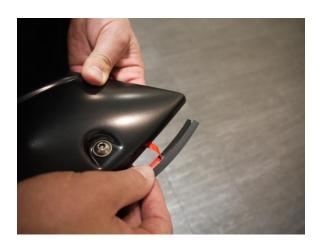
**STEP 1:** Attach the included rubber seal to the Fender Flares. Peel back 2" of the adhesive backing and position on the Fender Flare. Attach the seal to the Fender Flare, peeling back a few inches at a time. Ensure pressure is used to secure rubber seal to Fender Flare edge. Attach rubber seal along all areas where the Fender Flare contacts the vehicle body.
