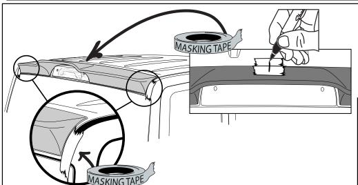
**STEP 3:** Place masking tape on roof aligning the edge of the masking tape to each end on the cab spoiler. Place masking tape centrally on the roof sheet metal and cab spoiler, mark line with a non-permanent pen to assist in positioning.
