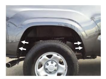
**STEP 12:** For models <u>without</u> factory installed Fender Flares, remove <u>only</u> the first (4) above indicated screws, from top to bottom of the fender, (2) each side, with a 10mm socket and retain for later re-installation.
