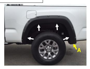
**STEP 11:** Hold Fender Flare on vehicle in the position of best fit. For models <u>with</u> factory installed Fender Flares, note where above marked holes in Fender Flare align with existing screws in the vehicle. Make special note of "A". Remove the EGR Fender Flare and remove the (4) above indicated screws from the factory flare with a 10mm socket. <u>DO NOT</u> remove the factory flare, the EGR Fender Flare installs directly over the factory flare.
