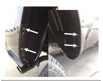
**STEP 12a:** Remove **ONLY** these (4) above indicated screws as mentioned in previous STEP 15, with a 10mm socket for models <u>without</u> factory installed Fender Flares. Leave all other remaining screws in wheel liner area. EGR Fender Flare will install directly over the remaining screws.
