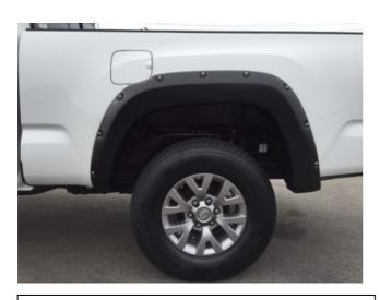
**STEP 13:** Re-Install Fender Flare in position of best fit, ensure that the rubber seal is sitting flat against the painted vehicle surface. Using (4) previously removed 10mm screws from STEP 14 or 15, reinstall at above mounting hole positions. Do not fully tighten screws at this stage.
