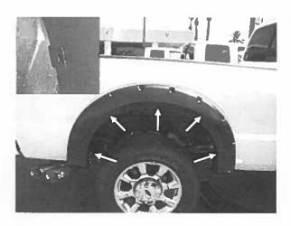
STEP 12: Place the Fender Flare onto the vehicle and fit into the correct position following the contours of the body. Use ten (10) of the .6mm clips (five 5 per side) to secure the Fender Flare to the body. Make sure the dimple in the clip securely attaches in the slot on the Fender Flare.
