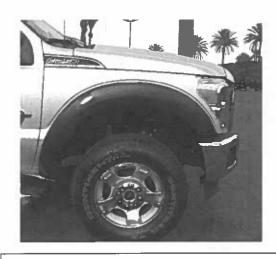
**STEP 7:** Place the Fender Flare onto the vehicle and fit into the correct position following the contours of the body. Ensure the slots in the part align with the holes in the fender from the previously removed 5.5mm socket head screws.
