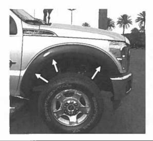
**STEP 8:** Reinstall the 5.5mm socket head screws through slots in the Fender Flare to the vehicle. Make sure the screws are securely engaged to the vehicle fender.
