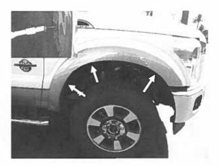
**STEP 6:** Remove all 5.5mm socket head screws and retain for installation of Fender Flares.
