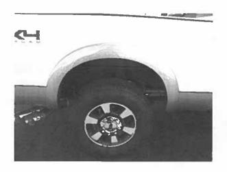
STEP 11: Clean the body areas where the Fender Flares will makes contact. Use the supplied alcohol wipe.
