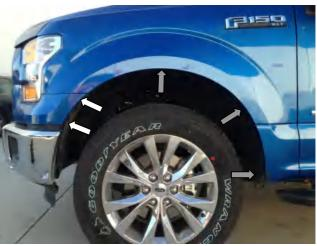
**STEP 2:** Locate three (3) 5.5mm bolts and two (2) 7mm bolt.
