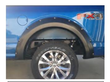
**STEP 7:** Repeat installation method for other side. Double check the front Fender Flares to make sure all bolts are tight and clips are securely fastened. Your installation is now complete. Do not use abrasive cleaners.
