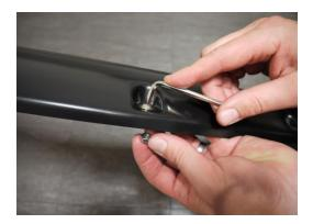
**STEP 1:** Attach the bolts and nuts to each Fender Flares using a 3/16" Allen key and a 10mm wrench/socket (wrench /socket and Allen key not supplied). Ensure inside of Fender Flares where the rubber seal is attached is clean, using the alcohol wipes provided. Wipe away any residue with a dry clean cloth.
