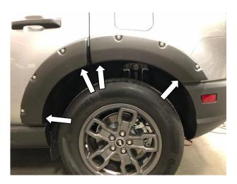
**STEP 11:** Continue to install the (4) remaining clips once fender flare is seated correctly. Be sure that the clips "snap" securely into the slotted hole of the fender flare. Once all clips have been installed, pull the exposed red tape liner and apply mild pressure to adhere properly to the vehicle.
