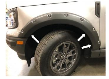
**STEP 7:** Continue to install the (3) remaining clips once fender flare is seated correctly. Be sure that the clips "snap" securely into the slotted hole of the fender flare. Once all clips have been installed, pull the exposed red tape liner and apply mild pressure to adhere properly to the vehicle.
