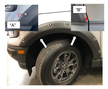
**STEP 6:** Pull red tape liner back 1-1/2", front and back of the Fender Flare, as shown in images "A" and "B" above. Place the Fender Flare onto the vehicle and fit into the correct position following the contours of the vehicle body. Use 2 of the retaining clips provided to secure the Fender Flare to the body starting at the positions pointed out above. Be sure the clips "snap" securely into the slotted hole of the Fender Flare.
