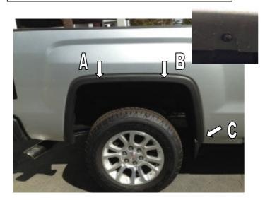
**STEP 9:** Place Fender Flare on the vehicle into the position of best fit. Note where the slots in Fender Flare at positions **A** and **B** align with the existing screws in the vehicle wheel arch molding. Also note where the slot in the Fender Flare aligns with the front mud flap deflector, position **C**. Remove Fender Flare. Remove the existing vehicle screws in location **A** and **B** using #15 Torx head screwdriver. Maintain screws for re-install.
