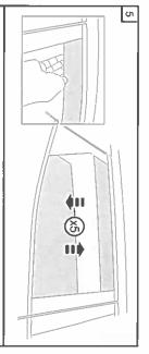
of the rubber window channel. Pull the bottom of the Window lowering the window a minimum of 5 times to help seat the Visor outwards at the rear of the part while raising and Ensure the Window Visor is located in the outermost section Window Visor into the rubber window channel
