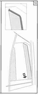
window channel, as shown Fit the front section of the Window Visor into the rubber
