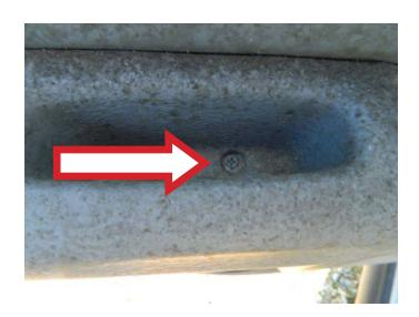
**STEP 2:** Using a pic or small flat-blade screwdriver, remove the cover exposing an interior door trim panel attaching screw. Once the cover has been removed, use a Phillips head screw driver to remove the interior door trim panel attaching screw.
