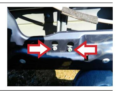
**STEP 3:** Loosely mount the top of the window regulator into position.
