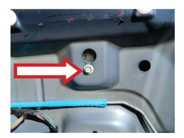
**STEP 13:** Once the window regulator attaching hardware has been removed, remove the window regulator assembly through the access hole.
