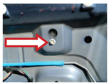
**STEP 4:** Once the window regulator has been put into position, tighten the window regulator attaching bolts.
