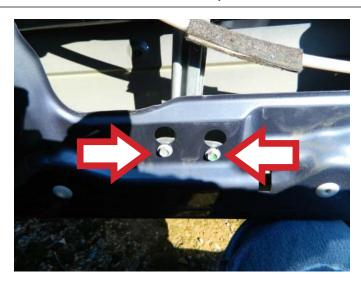
**STEP 12:** Remove the upper regulator attaching bolt.
