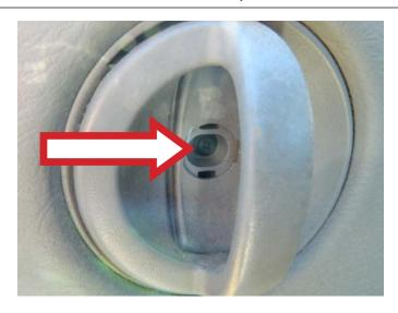
**STEP 12:** Install the interior door trim panel door pull retaining screw.
