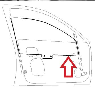
Be sure to check for gaps and to ensure that the weather-stripping did not fold underneath the window glass at any point of the window glass run channels.
