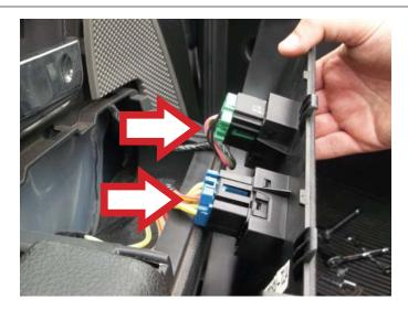
**STEP 9:** Once you have verified that the interior door trim panel retainers have been removed, lift the interior door trim panel in an upward motion to release the pre-molded retainers on the backside of the interior door trim panel. **NOTE:** This vehicle does not use a traditional interior trim retainer. Failure to lift the interior door trim panel completely from the door will result in damage to the interior door trim panel.
