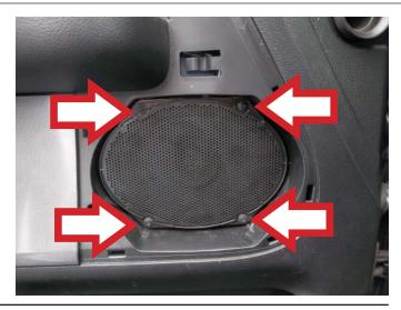
**STEP 6:** Once the speaker retaining screws have been removed, disconnect the door speaker.
