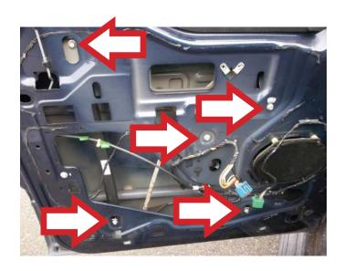
**STEP 15:** Once the window regulator attaching screws have been removed, remove the window regulator through the main access hole.
