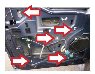
STEP 3: Connect the window lift motor.
