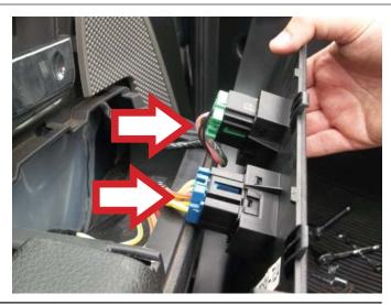
**STEP 10:** Attach the power switch assembly onto the interior door trim panel.
