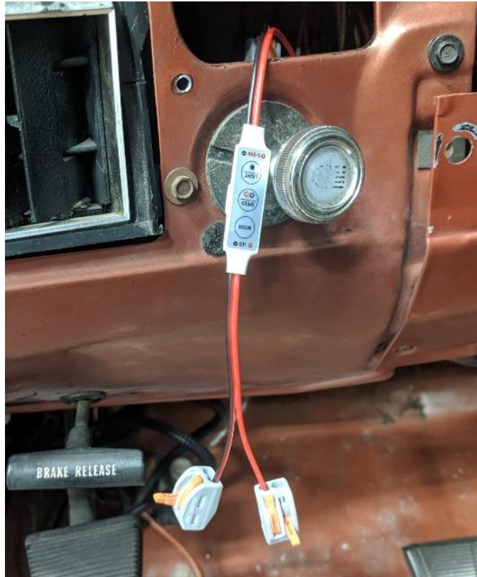
Figure 13 – Install Connectors to LED Dimmer
