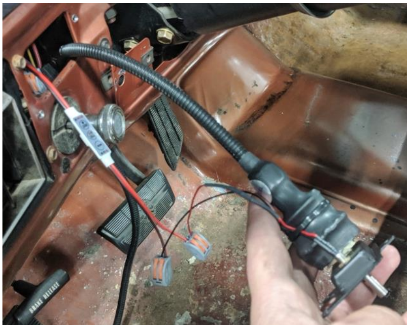
Figure 14 – Connect LED to Dimmer
