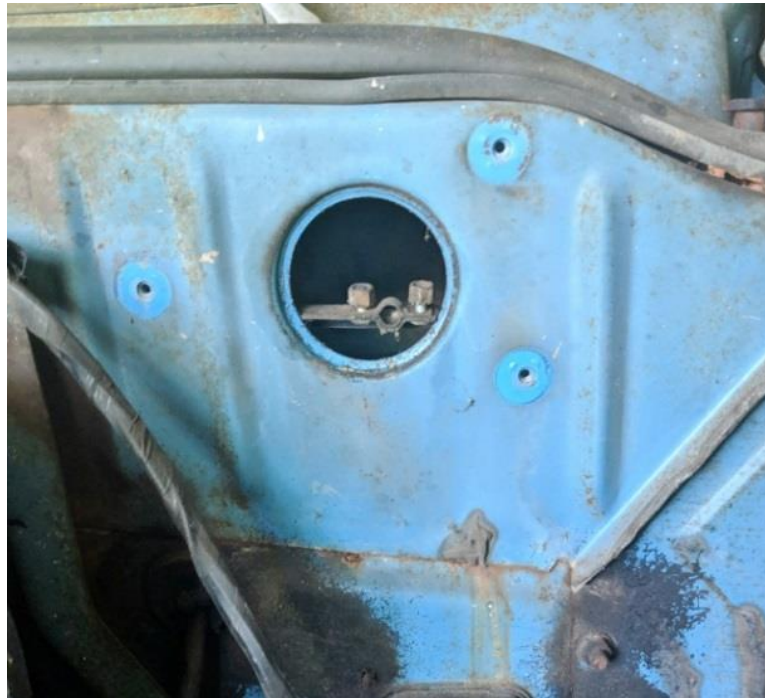
Figure 3 - Remove Stock Wiper Motor
