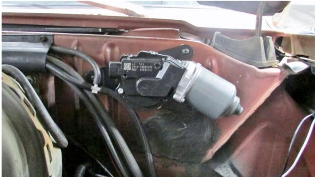
Figure 4 – Attach Wiper Motor to Firewall
