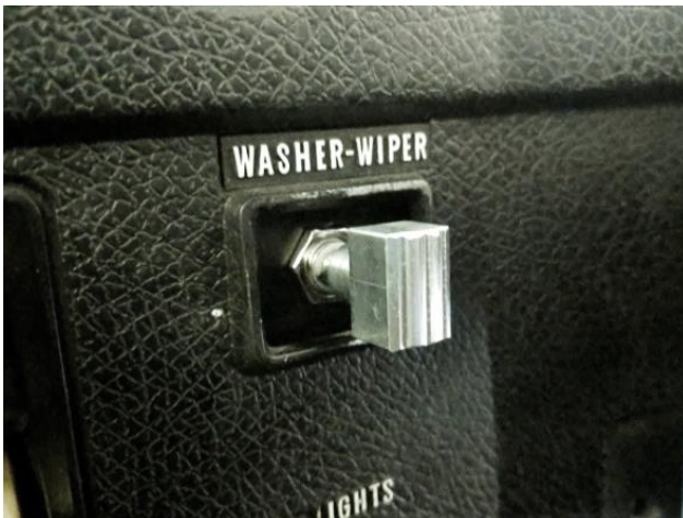
Figure 20 - Install Wiper Knob (1973-74)
