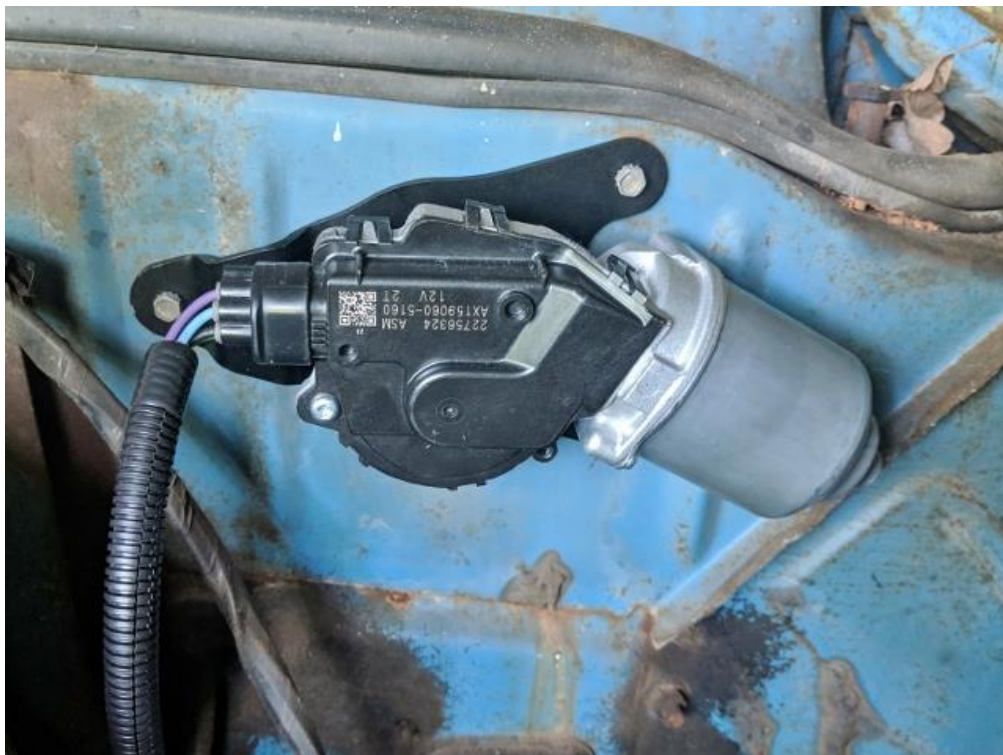
Figure 23 – Install Wiper Motor Harness
