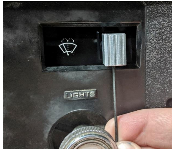
Figure 21 - Install Wiper Knob (1978-83)
