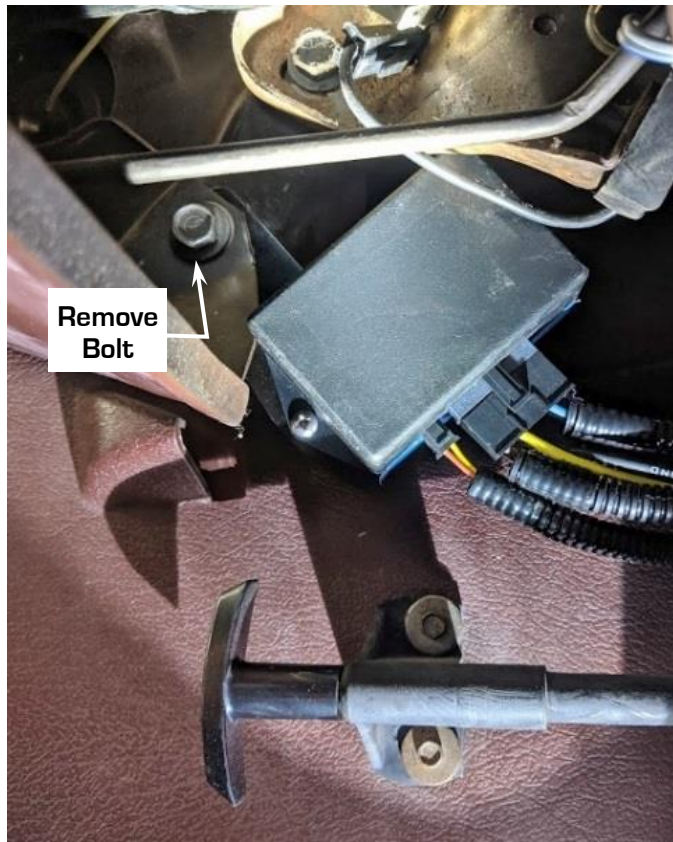
Figure 25 - Mount Control Module
