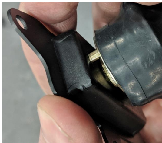
Figure 10 – Insert Wiper Switch into Light Box
