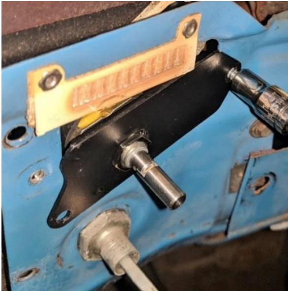
Figure 18 - Install Wiper Switch (1973-74) 83)
