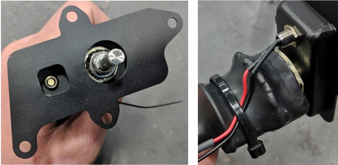
Figure 11 - Tighten Wiper Switch Assembly
