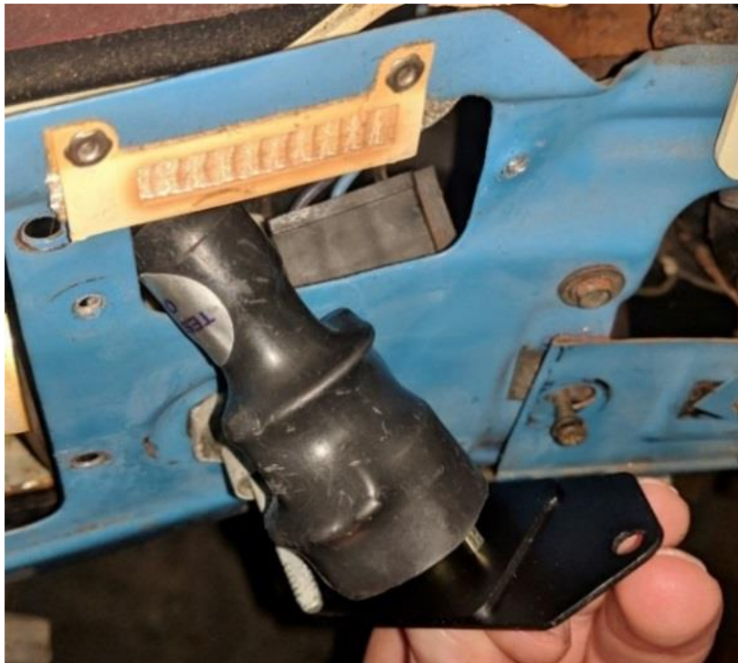
Figure 17 - Install Switch Adapter Plate (1973-74 shown)
