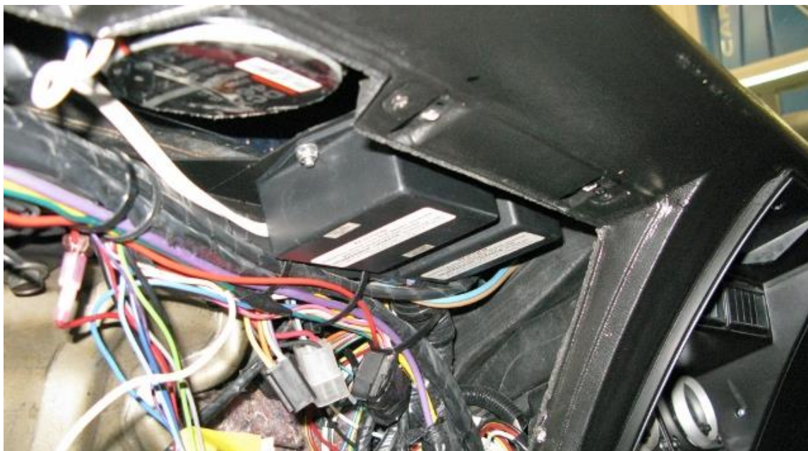
Figure 16 - Mount Wiper Module (Headlight Module also Shown)
