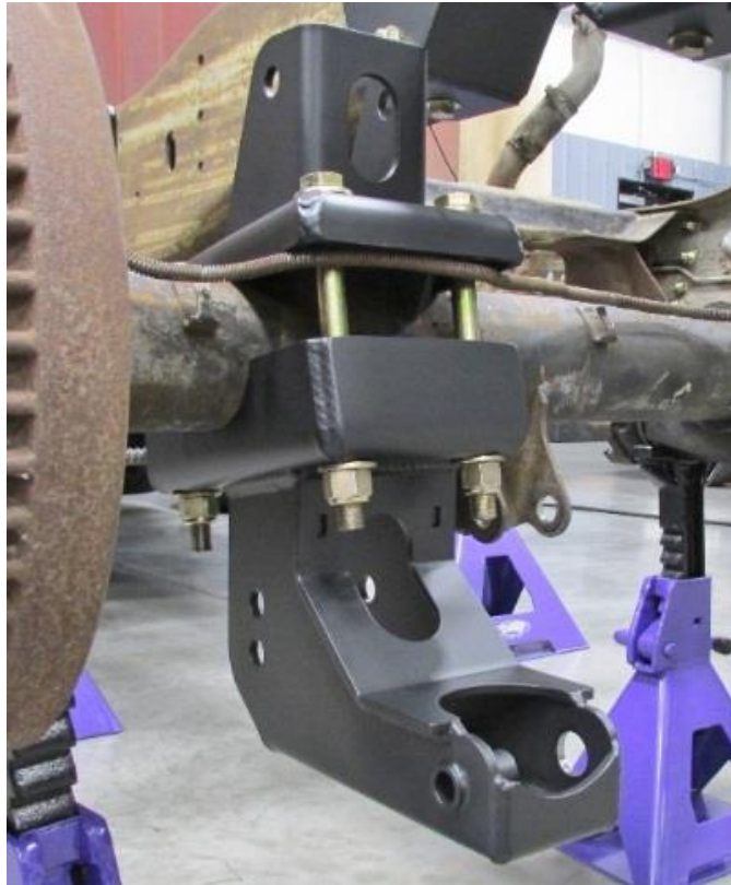
Figure 23 – Install Upper & Lower Axle Bracket (LH, Driver Side)
