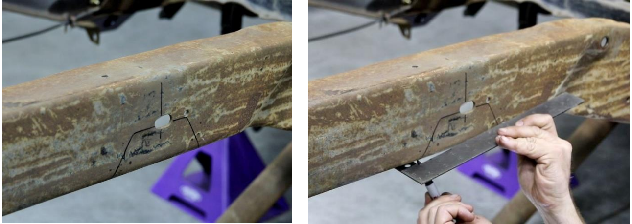
Figure 7 - Trace Frame Notch Cutout
