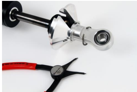
Figure 7 – Removing the Snap Ring
