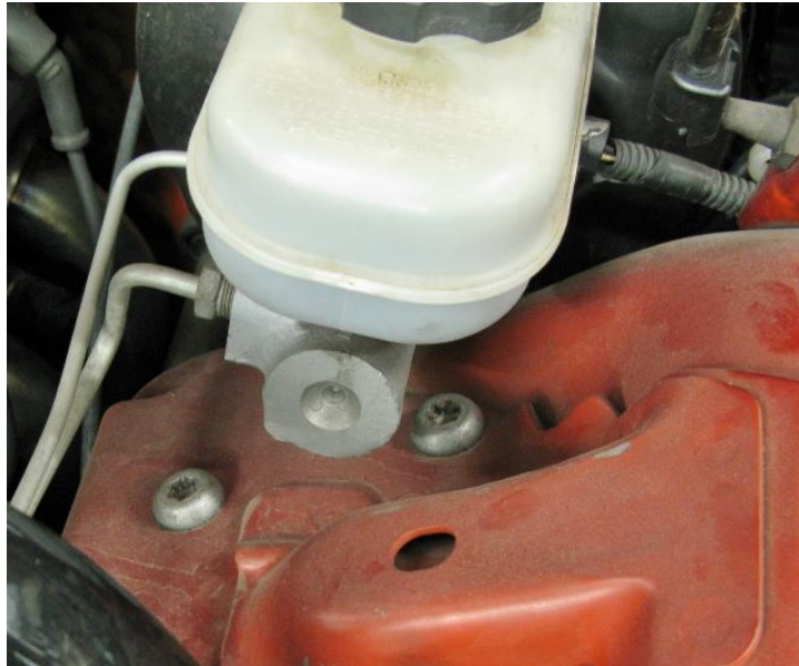
Figure 2 - Remove Torx Bolts
