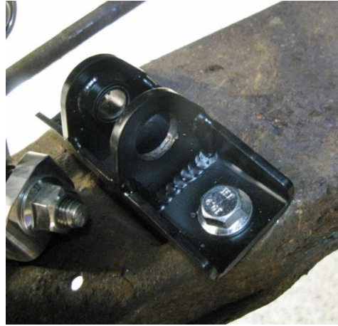
Figure 6 – Install Lower Shock Mount
