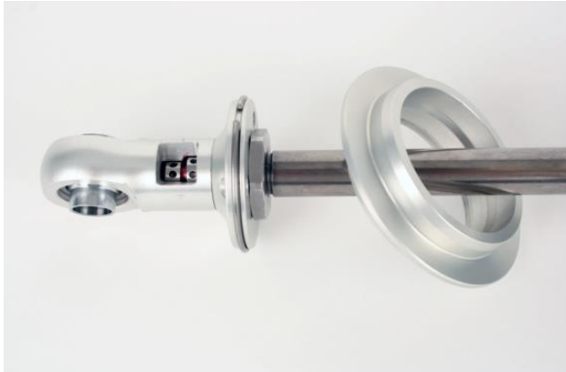
Figure 9 - Removing the Upper Spring Seat Ring
