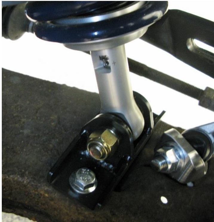
Figure 12 – Install Lower Shock Bolt
