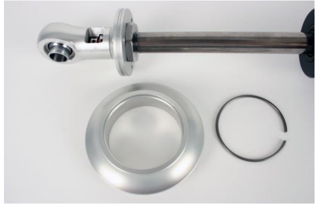
Figure 10 - Upper Spring Seat & Retaining Ring
