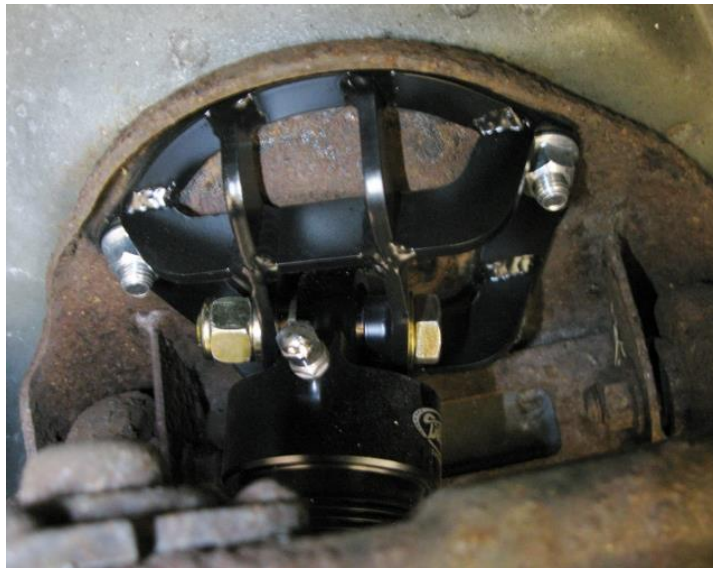
Figure 11 - Install Upper Shock Bolt
