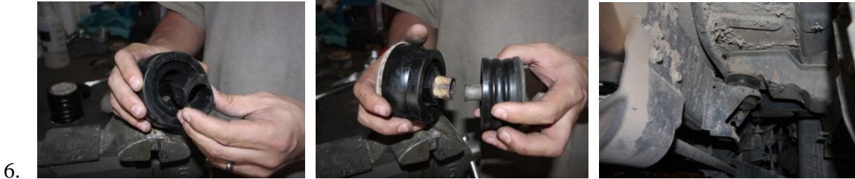
Figure 5: Body Mount location 2, A-Pillar. Use Body Cab Mounts M02544 (top) M02546 (bottom) , and insert M02542 (middle.) The insert will go into Cab Mount M02544.
