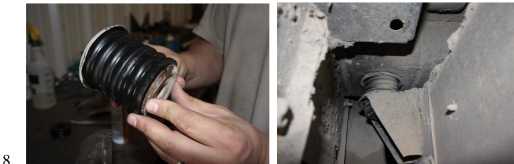
Figure 7: Body Mount location 4, C-Pillar. Use Cab Mounts M02342 (Top) and M02344 (bottom)
