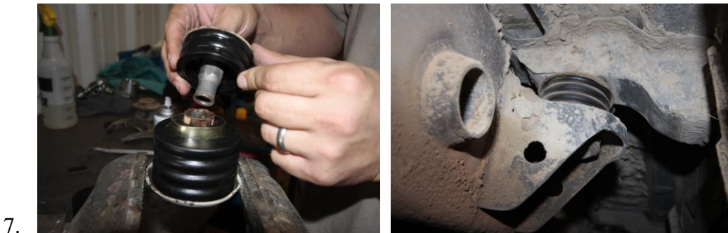
Figure 6: Body Mount location 3, B-Pillar. Use Cab Mounts M02545 (Top) and M02543 Bottom
