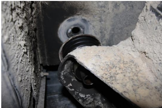
Figure 1: Loosen and remove the bolts at all locations, only do one side at a time. When the bolts are removed you will want to raise the side of the body that you are working on and remove the mounts. Keep track of which mounts came out of which location.
