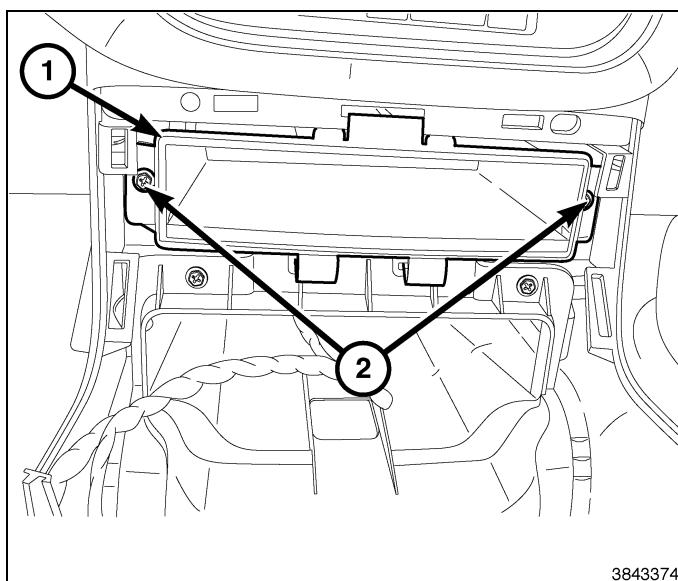
87. Obtain the kit supplied DVD power harness (1) and using a fishtape or equivalent, feed the harness through the front overhead console opening in the headliner. Route the harness down the A-pillar into the instrument panel and across to the center stack area.
