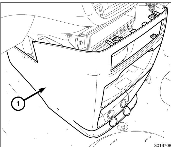
79. Remove the two fasteners (1) from the storage bin (2).
