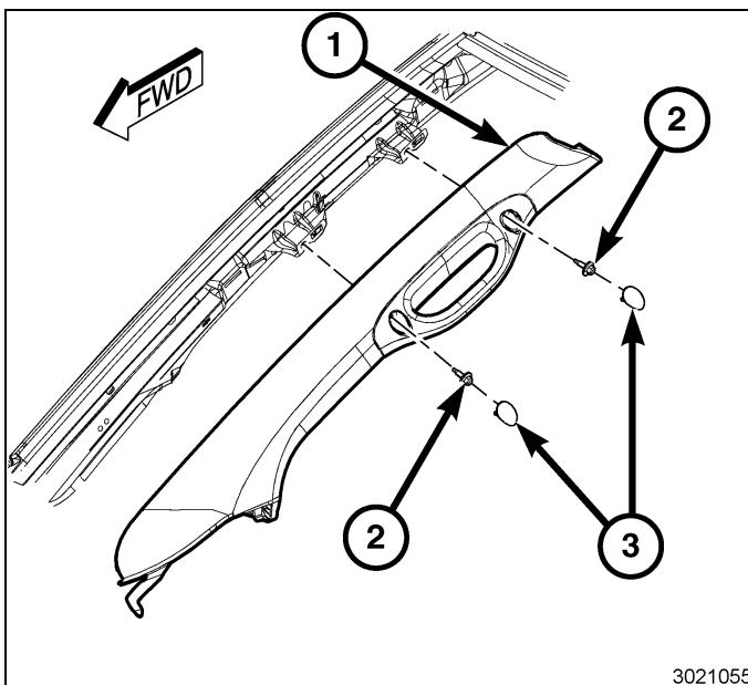
54. Disengage the visor (1) from the visor support.
