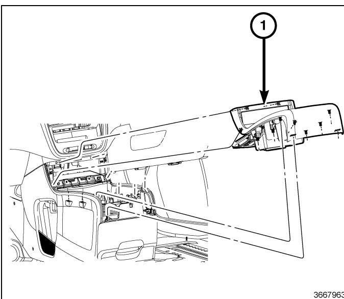
83. Rotate the upper console bezel (1) and disconnect the wiring harnesses (2).
