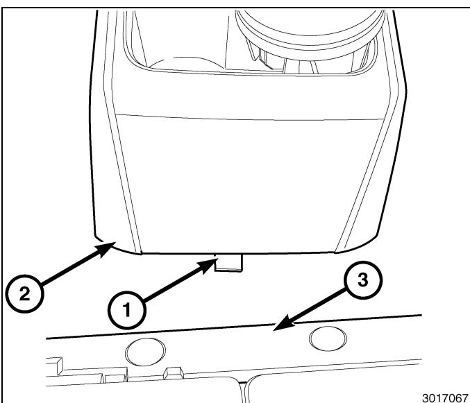
77. **Models equipped with base or premium floor consoles**, remove the four plastic retainers that secure the instrument panel bin (1) to the instrument panel.
