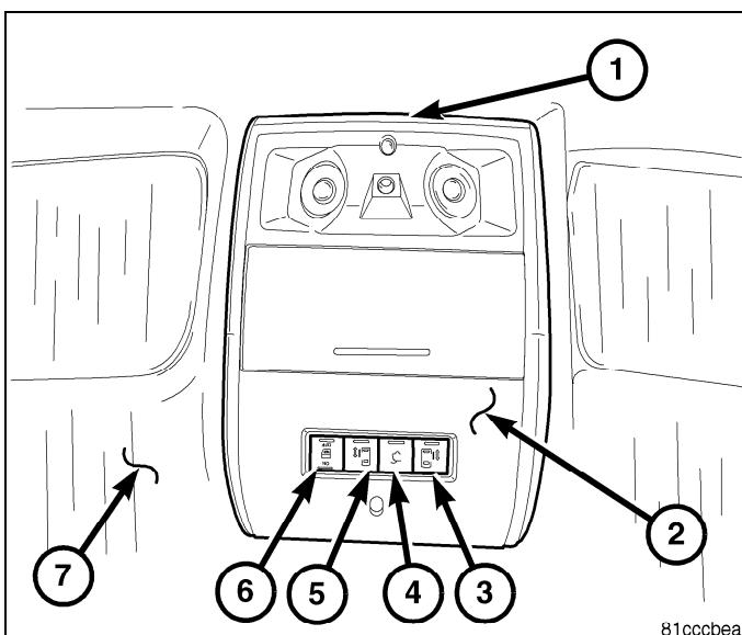
47. Lower the overhead console far enough to access the wire harness connectors.
