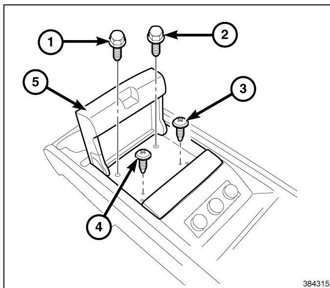
12. **Dual screen kit installation**, open the rear storage bin (5) on the overhead console.
