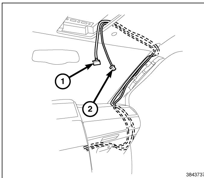
89. Using fishtape or equivalent, route the DVD power harnesses (1, 2) through the opening in the front overhead console cavity and route rearward.
