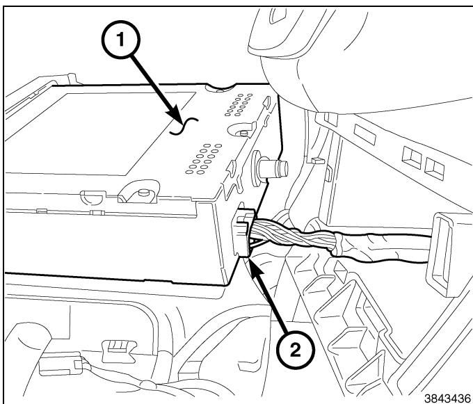
117. **Models equipped with full floor console**, install the fasteners (2) securing the DVD player to the instrument panel. Tighten the fasteners securely.
