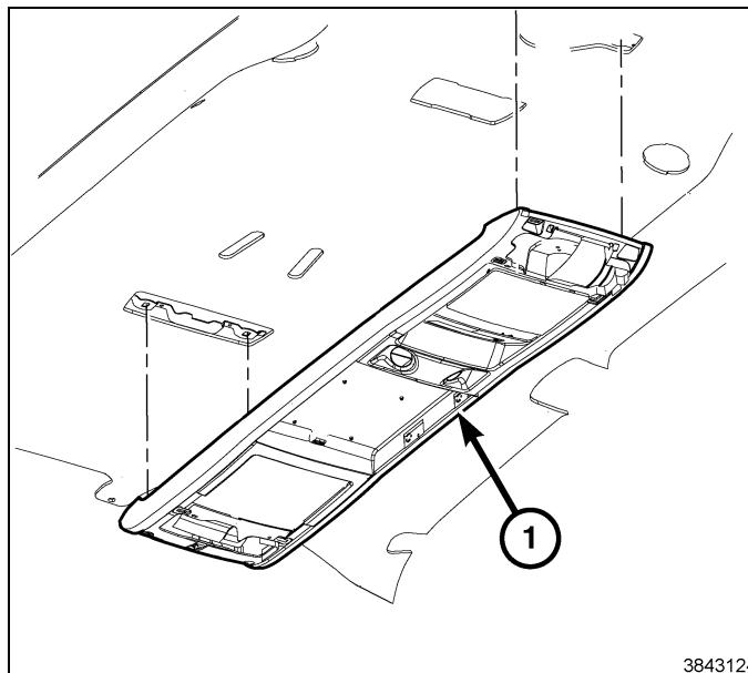
9. Place the overhead console face up on a clean work-bench.
