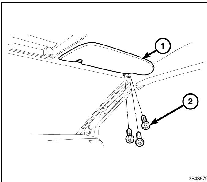
56. Remove the fastener (2) securing the visor support (1) to the vehicle. Remove the visor support (1).
