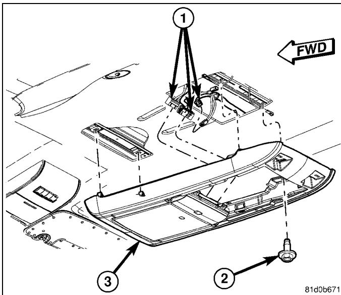
18. **Single screen kit installation into third row console**, use a trim stick or equivalent, gently pry down on the overhead console bezel (2).
