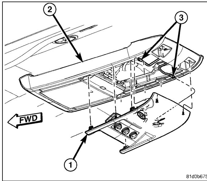
16. Remove the two screws (2) holding the rear of the overhead console (3).
