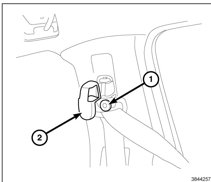
97. Using a trim stick, pry tool or equivalent, remove the upper C-pillar trim panel (1) from the driver side of the vehicle.
