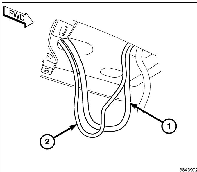
90. Continue routing the appropriate harnesses (2, 3) rearward to the rear overhead console area where the vehicle harness (1) is present.
