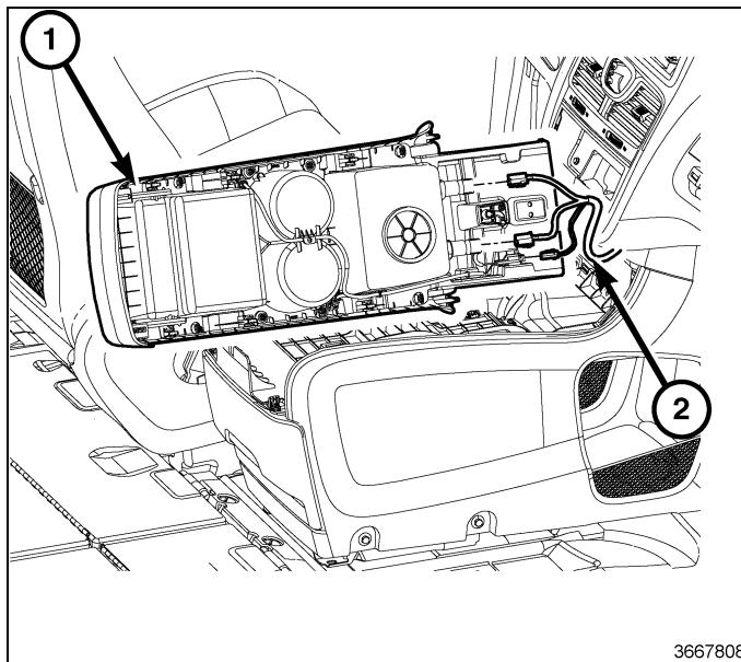
85. Remove the two fasteners (2) from the storage bin (1).
