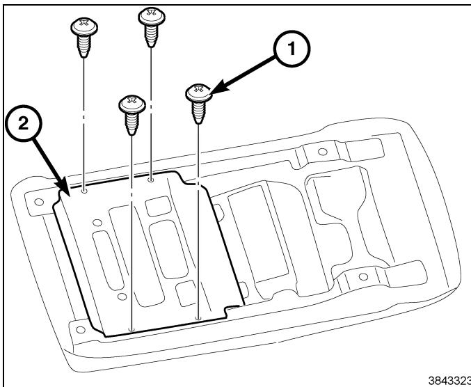
43. **Single screen kit installation into third row console**, turn the overhead console over and position the retaining bracket (2).
