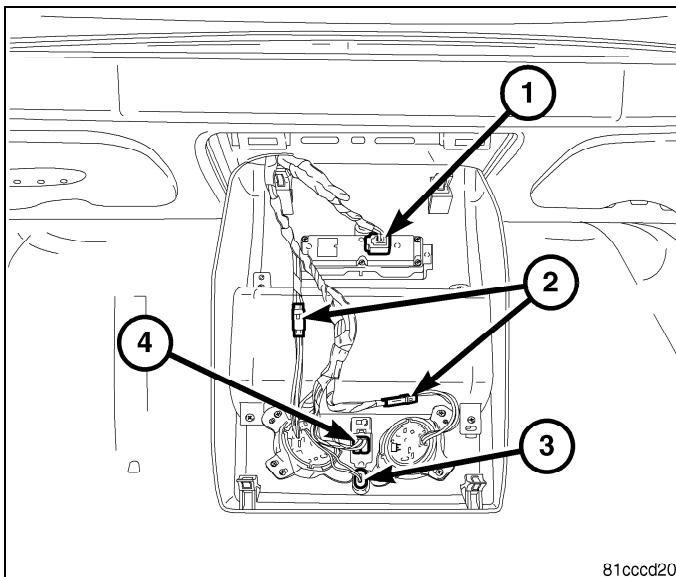
50. Using a small pry tool or equivalent, remove the fastener covers (3) from the A-pillar trim panel (1).
