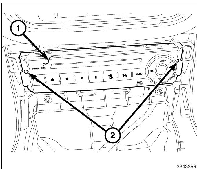
119. **Models equipped with base or premium floor consoles**, install the fasteners (2) securing the DVD player to the instrument panel. Tighten the fasteners securely.
