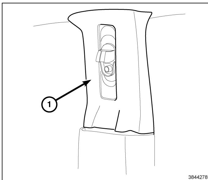
98. Using a trim stick, pry tool or equivalent, detach the auxiliary power bezel (1) located on the driver side quarter trim panel.
