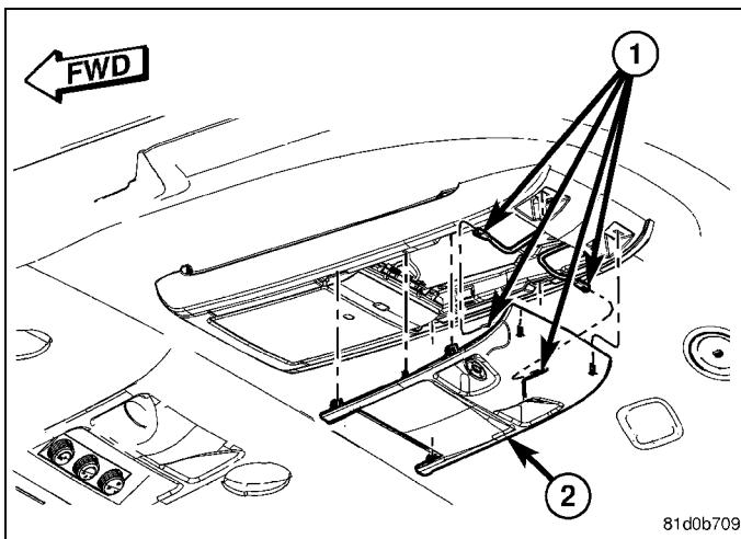
21. Remove the two screws (2) holding the rear of the overhead console (3).
