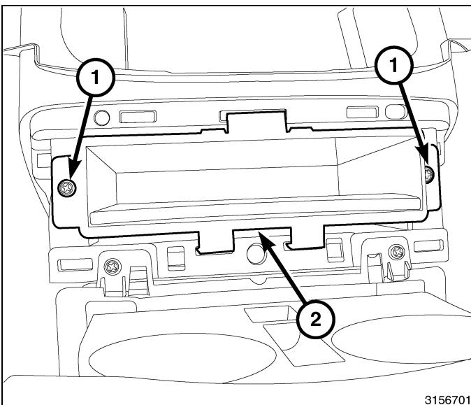
81. **Models equipped with full floor console**, using a trim stick or equivalent, pry around the perimeter of the upper console bezel (1) to disengage the retaining clips.
