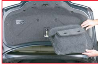
Align and install Pocket Pods™ using provided mounting components
