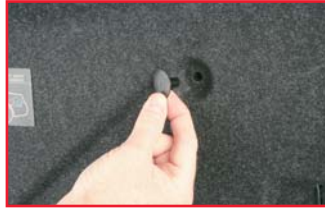
If required, remove specified clips/fasteners inside trunk lid
