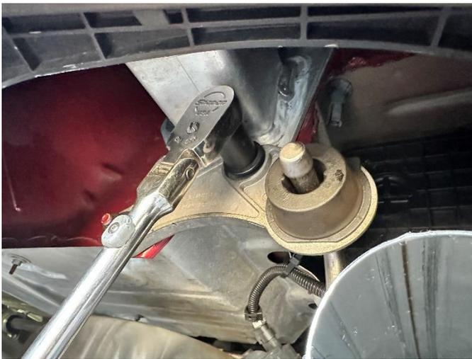
**25. (CARBON TIPS ONLY)** Locate the stock hanger grommet assembly mounting hardware from **REMOVAL STEP 4** and start them by hand onto the mounting studs. Tighten the hanger grommet assembly hardware using a 15mm socket and 3/8" ratchet. Repeat **INSTALL STEPS 22-25** for the driver side outer tip pipe assembly.
