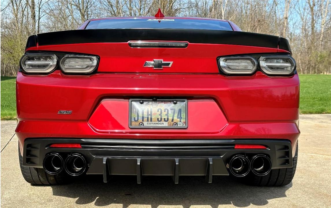
**34. (ALL VERSIONS)** Adjust the system accordingly, including the rear muffler rotation and overlap onto the stock exhaust, along with the tip and tip pipe depth and rotation, so that the tips are centered in the bumper valence. Check the position of all hangers to make sure they are properly seated within their corresponding grommets. Check clearances between the system components and chassis. Tighten all clamps to 45ft-lbs using the torque wrench and 15mm socket.
