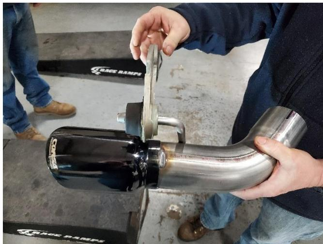
**12. (S.S. TIPS ONLY)** Install the stock hanger grommet assembly onto the tip hanger.
