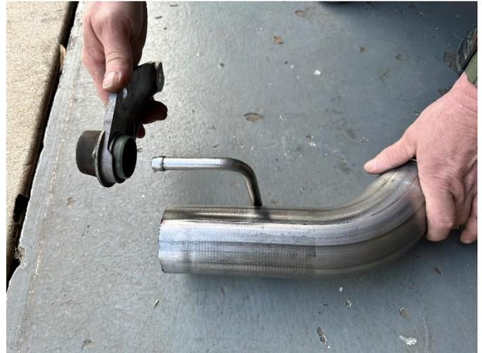
**22. (CARBON TIPS ONLY)** Locate the passenger outer tip pipe assembly and the stock hanger grommet assembly removed from the passenger side in **REMOVAL STEP 7**. Install the stock hanger grommet assembly onto the tip hanger.
