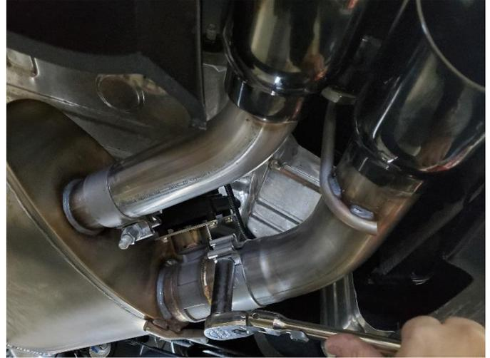
**20. (S.S. TIPS ONLY)** Snugly tighten the clamp securing the outer tip assembly to the muffler using a 15mm deep socket and 3/8" ratchet, leaving it loose enough for later adjustment.
