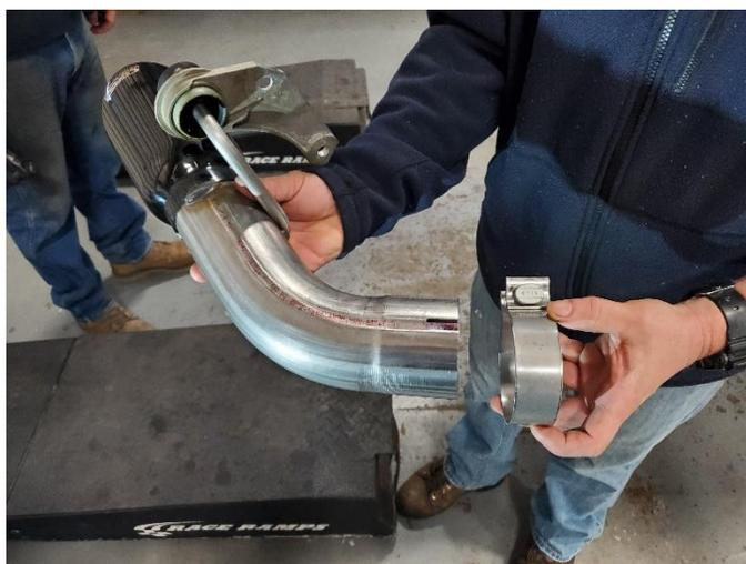
**13. (S.S. TIPS ONLY)** Locate one of the 3" clamps and slide the clamp onto the inlet of the outer tip assembly. Orient the clamp so the bolt is vertical with the nut towards the ground and the bolt towards the inside of the vehicle.
