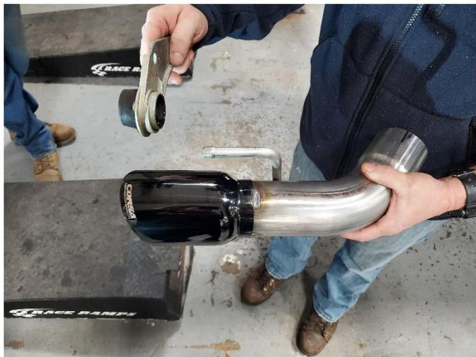
**11. (S.S. TIPS ONLY)** Locate the passenger outer tip assembly and the stock hanger grommet assembly removed from the passenger side in **REMOVAL STEP 7**.
