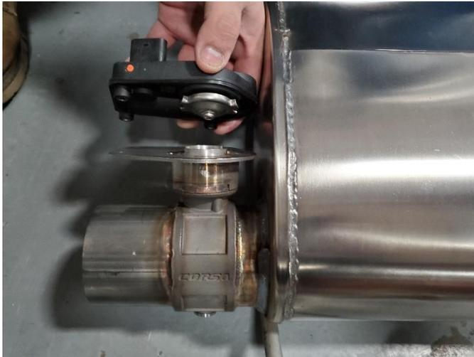
**1.** Locate the passenger muffler and the valve control unit removed from the passenger side of the stock muffler in removal step 9. Orient valve to match the rotation of the valve control unit as it was when removed from stock exhaust.
