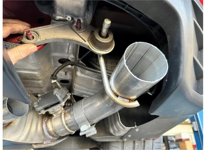
**24. (CARBON TIPS ONLY)** Install the stock hanger grommet assembly onto the mounting studs, then slide the outer tip pipe assembly inlet onto the valve outlet of the muffler.
