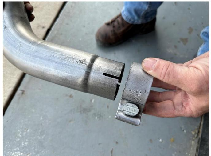
**26. (CARBON TIPS ONLY)** Locate the passenger inner tip pipe assembly and one 2.25" clamp and slide the clamp onto the inlet of the tip assembly. Orient the clamp so the bolt is vertical with the nut towards the ground and the bolt towards the outside of the vehicle.
