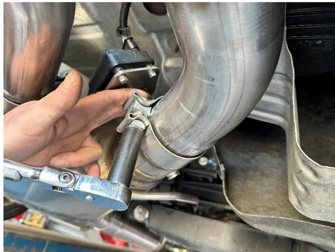
**28. (CARBON TIPS ONLY)** Snugly tighten the clamp securing the outer tip pipe assembly to the muffler using a 15mm deep socket and 3/8" ratchet, leaving it loose enough for later adjustment.
