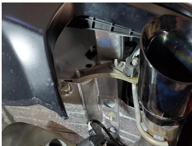
**14. (S.S. TIPS ONLY)** Install the stock hanger grommet assembly onto the mounting studs.
