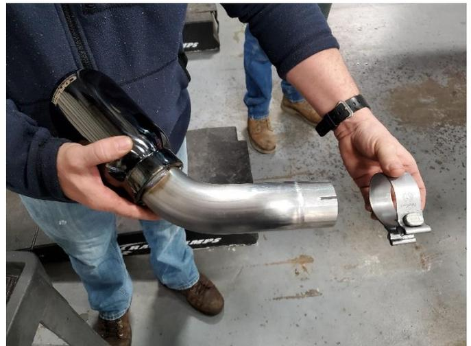
**18. (S.S. TIPS ONLY)** Locate the passenger inner tip assembly and one 2.25" clamp and slide the clamp onto the inlet of the tip assembly. Orient the clamp so the bolt is vertical with the nut towards the ground and the bolt towards the outside of the vehicle.
