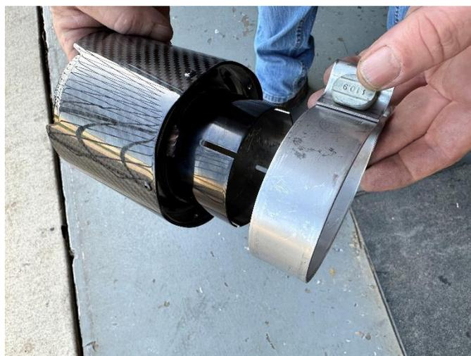
**30. (CARBON TIPS ONLY)** Locate one of the 4.5" outer carbon tip assemblies and one 3.0" clamp and slide the clamp onto the inlet of the tip assembly. Orient the clamp so the bolt is vertical with the nut towards the ground and the bolt towards the inside of the vehicle.
