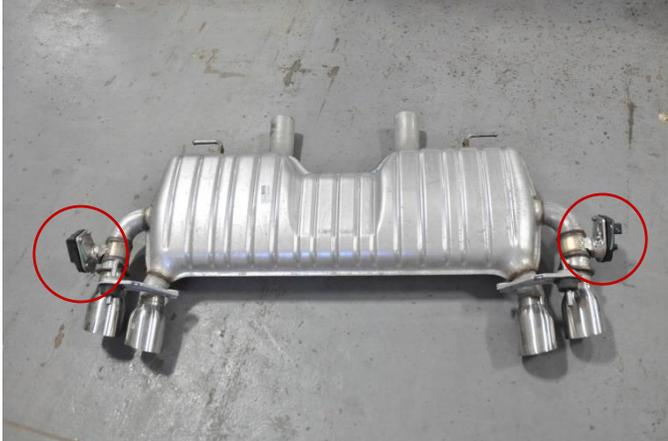
9. Remove the three screws securing each valve control unit to the outer stock tips using an 8mm socket and 1/4" ratchet. Label each unit with the position it was installed to make sure it goes back to the same location.
