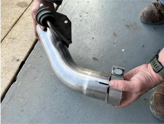
**23. (CARBON TIPS ONLY)** Locate one of the 3" clamps and slide the clamp onto the inlet of the outer tip pipe assembly. Orient the clamp so the bolt is vertical with the nut towards the ground and the bolt towards the inside of the vehicle.
