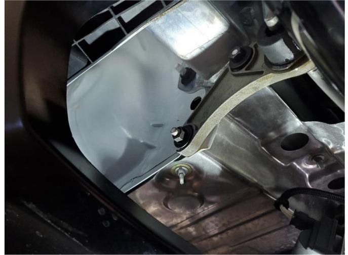
**16. (S.S. TIPS ONLY)** Locate the stock hanger grommet assembly mounting hardware from **REMOVAL STEP 4** and start them by hand onto the mounting studs.
