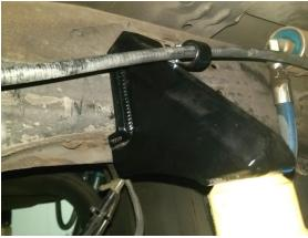
6. Install the Bump stop strike plates into the keyways on the U-Bolt plates on both sides. These plates should fit flush; if they contact a U-Bolt thread, use a cutoff wheel to trim the interfering U-Bolt. Once cleared, assemble plates (sloping to the rear) and install the provided 3/8" hardware and torque to 40lb/ft.
