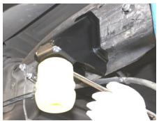
5. Using the provided self-tapping bolt and P-Clamp, secure the E-Brake cable to the existing hole on top of the Driver's side bump stop drop bracket. Don't over torque a quarter turn past tight will be sufficient.
