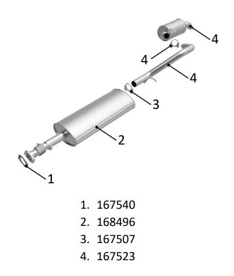
(Carefully read all instructions before installation) Disconnect the vehicle's battery before removal of the OEM exhaust system. This will prevent electrical accidents and will reset the computer if it applies to the vehicle. Remove existing exhaust system from the vehicle. Only remove parts that will be replaced. Clean existing flange with a wire brush to ensure proper sealing.
