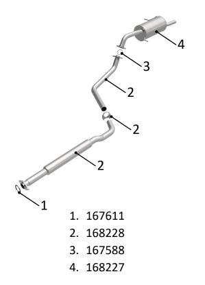
(Carefully read all instructions before installation) Disconnect the vehicle's battery before removal of the OEM exhaust system. This will prevent electrical accidents and will reset the computer if it applies to the vehicle. Remove existing exhaust system from the vehicle. Only remove parts that will be replaced. Clean existing flange with a wire brush to ensure proper sealing.
