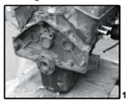
Remove the old trans so that all you have left is a bare engine block and crankshaft showing (photo 1)
