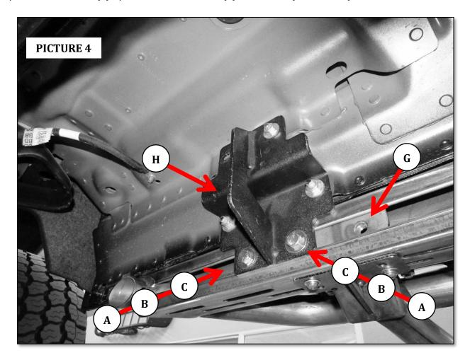
**Step-5** Align the running board with the vehicle and tighten all bracket and side step nuts and bolts,. Repeat the above steps to install the driver side brackets and running board. Remember to check and retighten the nuts and bolts every six months.
