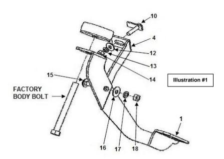
Step-3 Remove the passenger side middle body mount bolt, (Photo 3).
