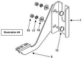
**Step-9** Attach the side step to each bracket using (1) U-bracket (2) 5/16" hex bolts (2) 5/16" lock washers and (2) 5/16" flat washers then align the side step with the vehicle and tighten all side step and bracket nuts and bolts, **(Photo 7 & 8)**.
