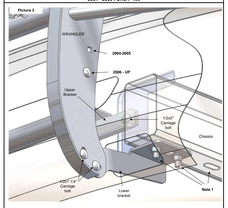
Diagram shows lower bracket installation for NON TOW HOOKS vehicle, if TOW HOOKS exist, please use bolt's vehicle remaining tow hooks as before.
