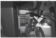
Figure 1 3. Pull out the bundle of wires from the conduit that lead to the **Blue** connector unplugged in **Step #2** shown in Figure 2.
