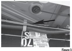
**12.** Continue routing 4-Flat along the factory wire harness to front of vehicle securing it along the way with cable ties. Route up into the engine compartment along factory wiring harness shown in **Figure 4.**
