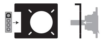
Plug the combination harnesses' trailer-style 4-way flat connector into the tow vehicle's 4-way flat connector. This connection will provide the tail lights, stop lights and turn signal functions. See below picture.
