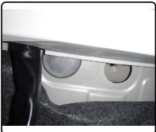
2. Remove tow hook by removing hardware through access holes in trunk pan than remove hardware from underneath vehicle. Put tow hook and hardware in bag and return to vehicle owner.
