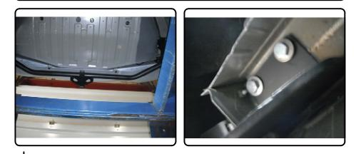
4. Loosely install bolts and washers through access holes in trunk pan. Then torque all M12 hardware to 65 ft-lbs
