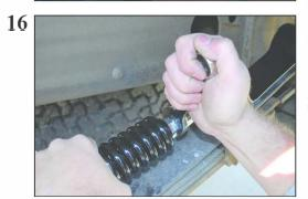
16) Finally, jam one of the two nuts located in the center of the threaded rod hard against the coil spring, then follow with the second nut and jam against the first.
