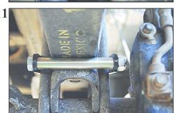
11) Next attach the nylon nut and tighten.
