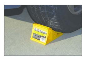
1) Before starting the installation make sure the vehicle is on a level surface, then place wheel chocks on both sides of the front wheels.
