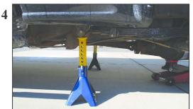
4) Next raise the rear of the vehicle with the jack sufficiently to place jack stands on both sides of the vehicle. As the vehicle has rear leaf springs, the ideal place to position the stands is under the front eye of the leaf springs, connected to the fixed shackles, as illustrated. With the floor jack still under the differential, next remove the rear wheels. With the lug nuts now loosened, this will make the removal a lot easier.
