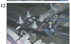
12) When fitting to some Ford vehicles where the U bolts are located around the axle and have a hold down plate on top of the leaf springs, the axle connecting bracket must be located the same way as in illustration (10) also with the bolt and spacer directly under the leaf springs (11).
