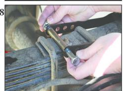
8) Next remove the nut, bolt and spacer. The bracket should now hang astride the leaf spring pack and U bolts.
