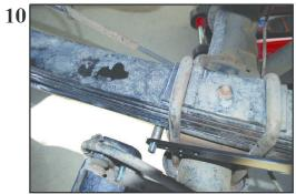
10) With the axle bracket now in positioned under the leaf springs, insert the connecting bolt and spacer as shown in the illustration.
