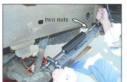
14) Position the two nuts on the threaded rod as shown. Then use a ratchet fitted with a 12 mm socket on the head of the cap screw, and a 22 mm wrench on the lock nuts closest to the eye bracket at the end of the threaded rod. The two nuts come locked together when the kits are assembled at our factory. By holding the threaded rod stationary and turning the coil spring the gap between the coils will start opening.
