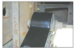
6) The RAS kit comes fully assembled out of the box. Remove one side and place it on top of the rear leaf spring with the eye bracket hook (C) facing the rear of the vehicle. Next position the eye bracket over the rear wrap eye of the leaf spring, as illustrated.
