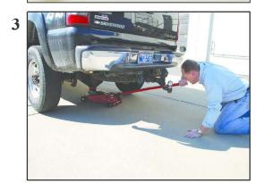
3) Position a floor jack of (the correct capacity for your vehicle) under the differential housing.
