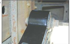
13) Before adjusting the coil spring to the correct tension, check to see that the eye bracket is in the center of the spring eye.
