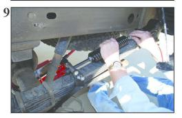
9) To lengthen the unit so the bolt spacer and nut can be located on the other side of the U bolt and under the bottom leaf spring. Start turning the coil spring with one hand and hold the threaded rod with the other.
