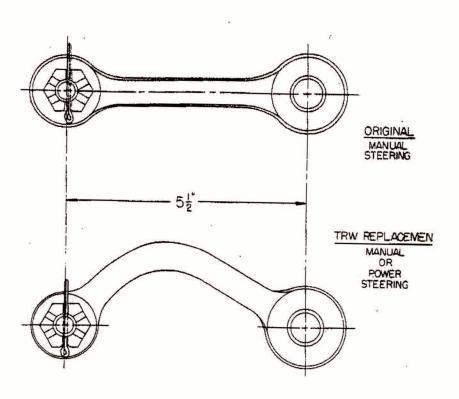
This TRW curved design idler arm replaces OEM idler arms for either manual or power steering applications.
