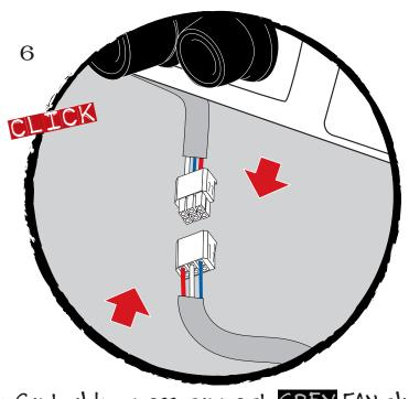
From Control harness connect GREY FAN plug into GREY corresponding Harness.
