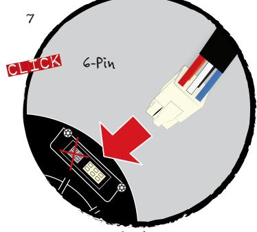
Connect Black Harness into Control 6 Pin Port on Evaporator.
