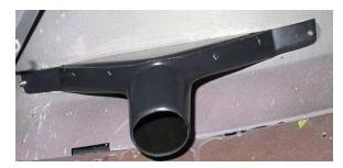
Locate the (2) defroster ducts and (4) #6 x % Black Phillips head screws, and attach as shown.
