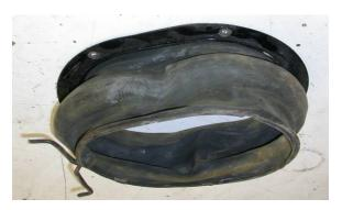
Remove and discard air inlet duct.
