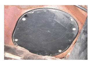
Locate the air Inlet Block Off Plate, and attach as shown using (4) #10 x 3/4" tek screws.
