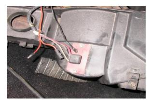
Disconnect electrical plug from resistor on the heater
