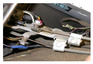
Remove cables from back of the control head. Retain original hardware for the cable clamps.
