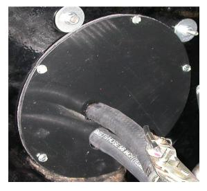
Locate firewall cover plate and using the (5) original screws Install cover.
