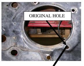
Route the longest Bowden cable through the original mounting hole shown
