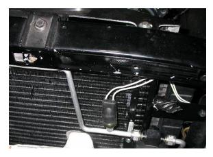
Attach liquid tube to drier using (1) #6 oring to And a drop of mineral oil and Tighten fitting.
