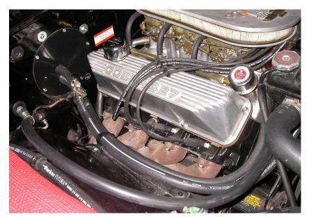
Locate #10 suction hose and (2) #10 o-rings add a drop of mineral oil to o-rings and attach hose to fitting on the evaporator end and route hose with the service port end to the compressor as shown.
