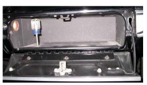
Install original Glove Box using original hardware as shown.
