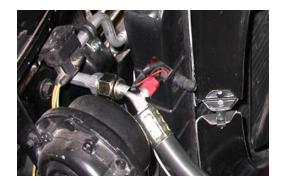
Attach the #8 discharge hose to compressor using (1) #8 o-ring and a drop of mineral oil. Route the other end of the #8 hose and attach to condenser fitting using (1) #8 o-ring and a Drop of mineral oil.
