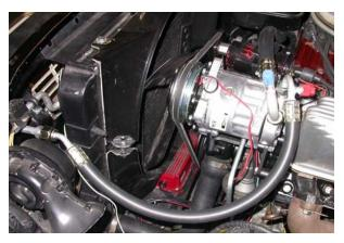
Install #8 discharge hose and (2) #8 o-ring and a few drops of mineral oil. Attach end of the hose with 45 deg fitting to the condenser fitting and end with the service port to compressor.
