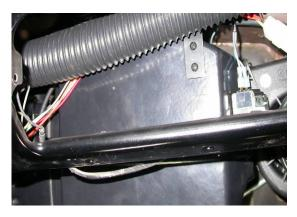
Route a/c wire harness from blower switch across the evaporator and plug in to blower motor connector.
