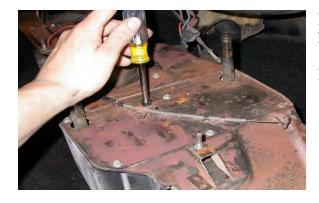
Remove control cable from center of O.E heater. Discard the cable.
