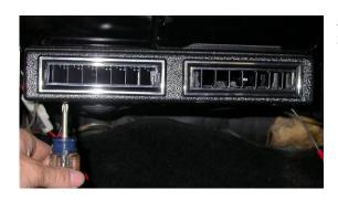
Attach center louver assembly to adaptor using (2) # 8 phillips screws.
