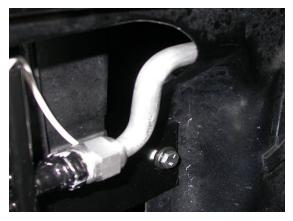
Install the discharge tube using (1) #8 oring And a drop of mineral oil and tighten fitting.
