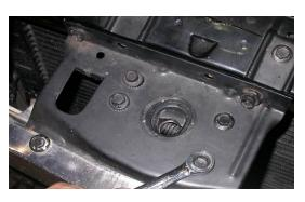
Remove and retain hood latch and mounting hardware as shown
