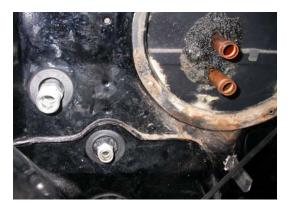
Insert heater Tubes and a/c tubes through hole in the firewall as shown.
