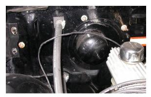
Remove the two heater lines from heater core.
