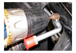
Attach (1) #8 clamp and (1) #10 Tek screw Install radiator cowl to hold liquid tube as shown.
