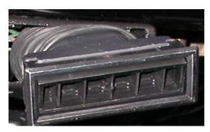
Attach duct hose to louver and snap louver into bezel.
