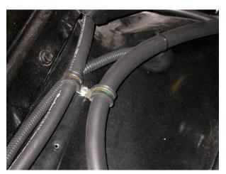
Install (1) #16 hose clamp and (1) #14 clamp on suction and liquid hose and attach to fender well using (1) #10 Tek screw as shown.
