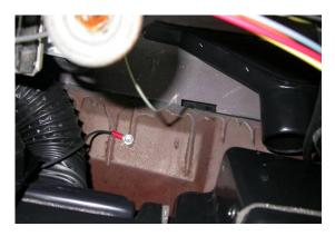
Attach black ground wire from wire harness to the body using (1) #10 Tek screw as shown.
