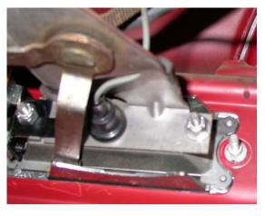
Plug the control head light connector into control head.
