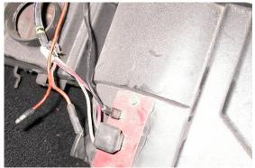
Locate black wire with spade connector that was attached to the original blower resistor. Cut off the connector and add a 1/4" male spade connector.
