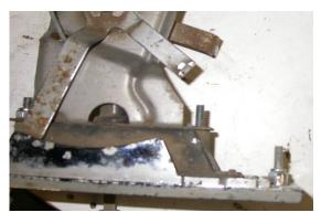
Remove and discard old blower switch from the original control head. Retain the hardware.
