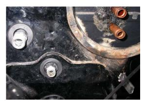
Drill a 11/16" hole  $\frac{1}{2}$ " lower than the evaporator drain tube.
