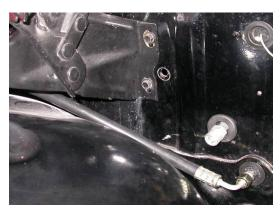
Route liquid hose along fender well to the evaporator fitting and attach using (1) #6 oring and a drop of mineral oil and tighten fitting.
