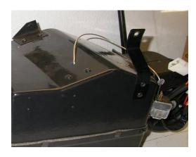
Locate the Top Front Mounting Bracket and (2) #8 x 3/8" Black Phillips Head Screws, and attach as shown.
