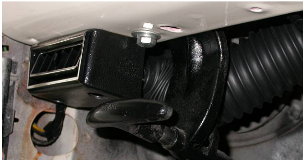
ATTACH LOUVER HOUSING TO DRIVERS SIDE OF THE DASH USING (2) #10 TEK SCREWS
