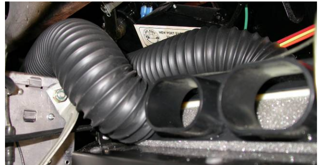
ROUTE 43" HOSE OVER RADIO AND OVER TO THE DRIVERS LOUVER
